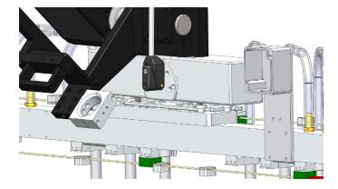
SR-56 quick-release mechanism shown with the tooling lock disengaged and the hand in load / unload position. Inserting the hand and turning the tooling lock will raise and secure the hand.
